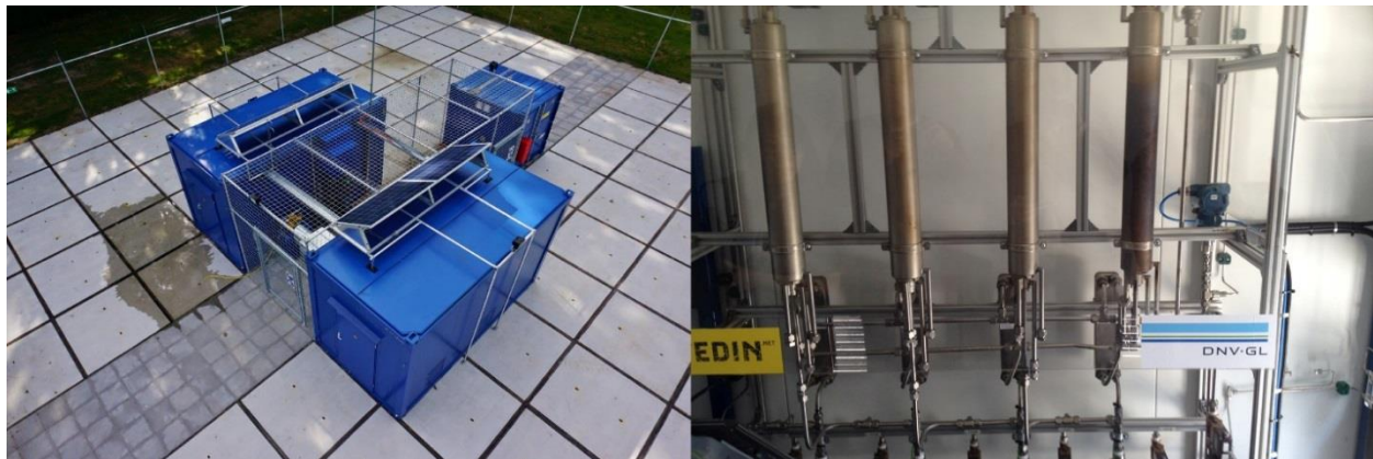
Figure 2: Small Power-to-Gas Unit with Close-Up of Methanization Reactors
